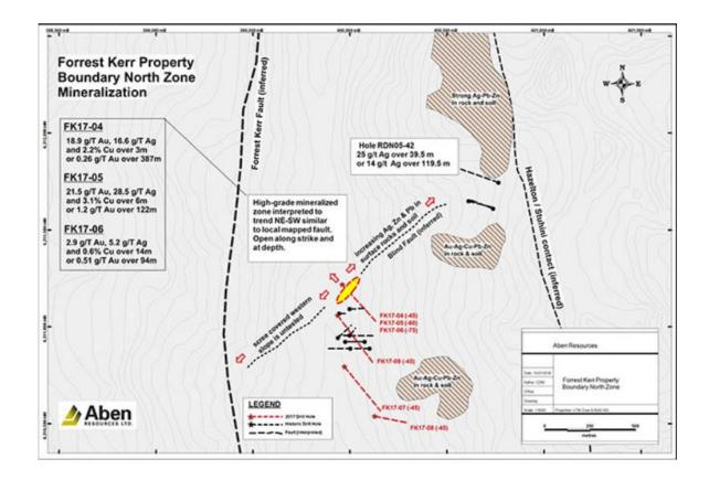
The goal of this year's 5,000m diamond drill program is to expand the mineralization at the Boundary North Zone. According to Aben, this part of the Forrest Kerr property hosts gold-silver-copper in rock and soil anomalies that span over 2 km by 4 km and remain relatively under-explored. The zone's mineralization remains open in multiple directions with numerous soil geochemical anomalies and geophysical targets yet to be drill-tested.
