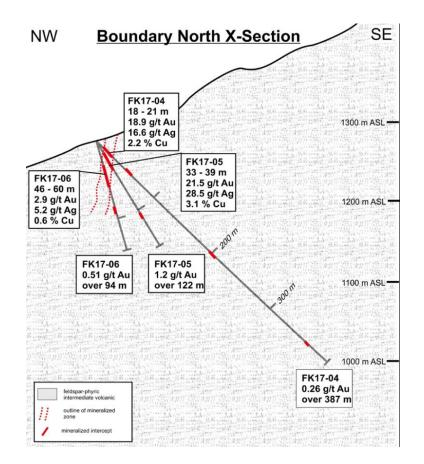
Last summer at Forrest Kerr, three separate drill holes, collared from the same drill pad and drilled in a fan pattern of 45, 65 and 75 degree dip, pierced a nearsurface high-grade zone of gold-silver-copper mineralization, in addition to broad intercepts containing gold-bearing quartz veins.
