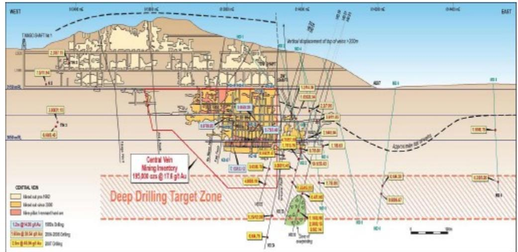
Figure 1. Longitudinal Section through Co-O mine
